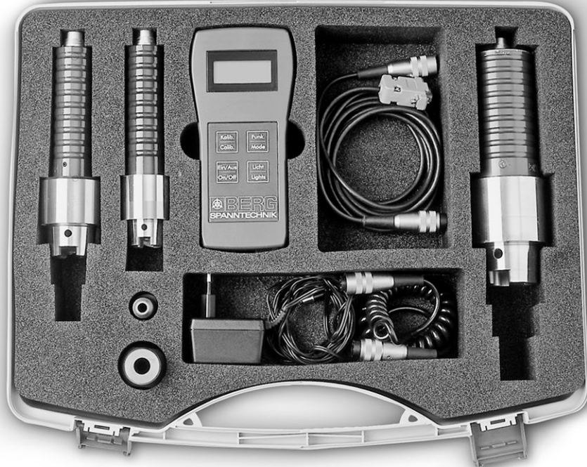
Example: Clamping force measuring system from Berg
